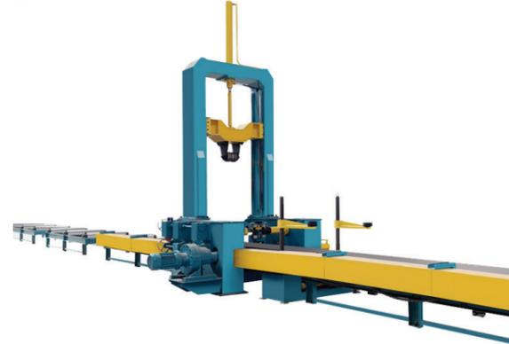
■ **H-Beam Assembly Machine (KHBA 1500)**
